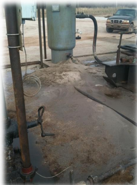
Sand Produced with Jet Pump
