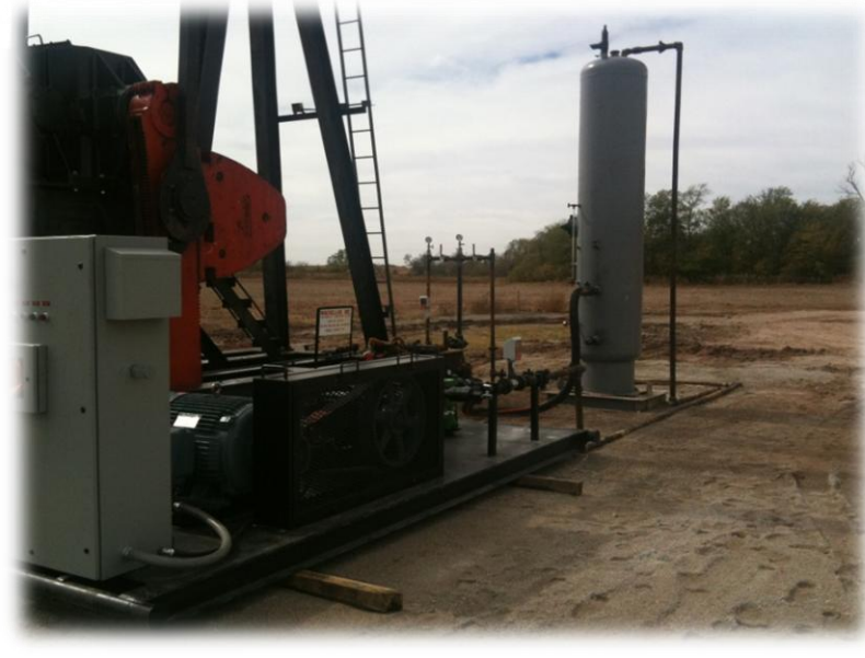
Diaphragm Pump Skid In Front of Pumping Unit
